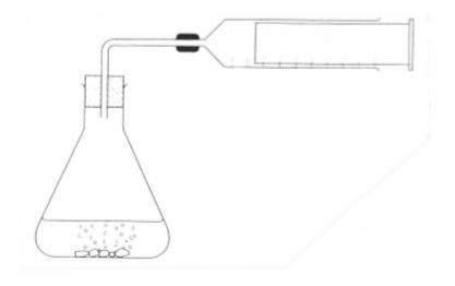
A 1.60 g sample of pure sulfamic acid was dissolved in water and then transferred to the conical flask. An excess of magnesium ribbon was added to the flask and the bung was quickly replaced.
